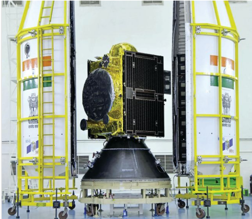
THE NVS-02 NAVIGATION SATELLITE being encapsulated into its payload ahead of its launch on Jan. 28, 2025.
